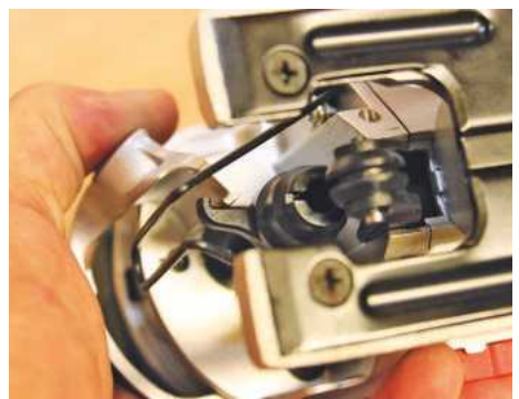
▲ An alloy front lever operates the blade swap function
